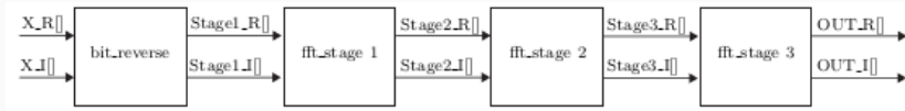
Figure 1: Dividing the FFT into different stages allows for task pipelining across each of these stages. The figure shows an example with three FFT stages (i.e., an 8 point FFT).
